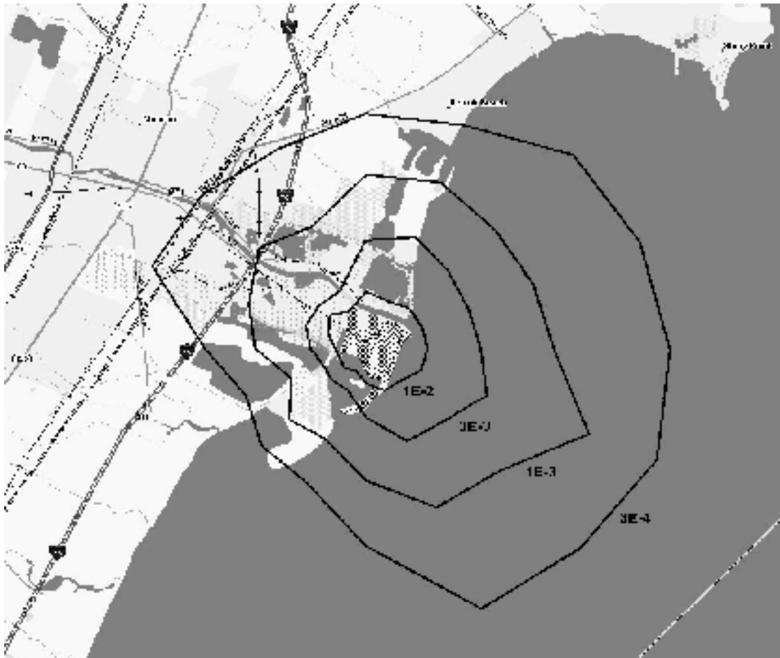
FIGURE 3 INDIVIDUAL ISORISK CONTOURS: ANNUAL FREQUENCY OF EXPOSURE TO ERPG-2 CONCENTRATION OR GREATER
